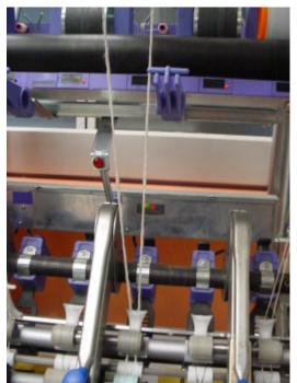
roving stop device as well. The detection is carried out either through a sensor at the pigtail or at the ring rail.
